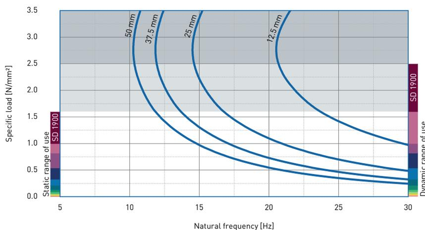
Natural frequency of a single-degree-of-freedom system consisting of a fixed mass and an elastic bearing consisting of PURASYS **vibrafoam** SD 1900 on a stiff subgrade.
